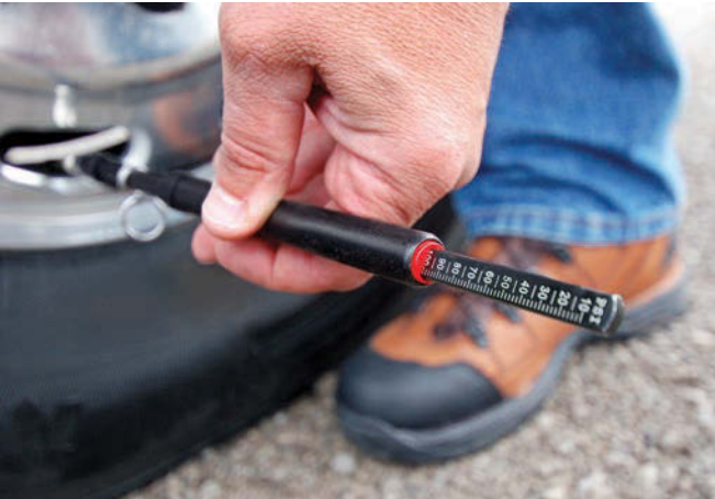
▲ For commercial vehicles, tire inflation should be based on scale weight by axle and the load/inflation chart for the appropriate tire size.
