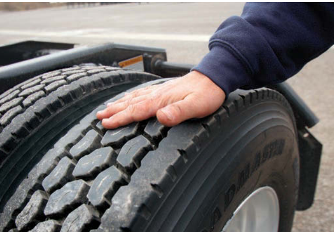
▲ Tires used on both paved and gravel roads, or even off-road, require a different tread design and cut/chip-resistant tread to give good service.
