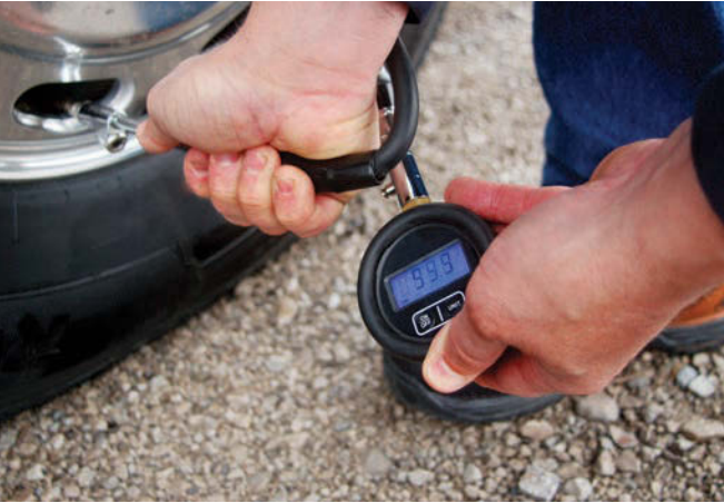
▲ Proper inflation is the single most important factor in extending tire life. (Photos courtesy of Cooper Tire and the Roadmaster brand)
