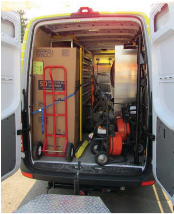
▲ A 50-gallon gas water heater and three General drain cleaning machines are kept near the rear doors for easy access. A 1,000-pound electric winch, made by Superwinch, helps technicians load and unload the heavy drain cleaning machines.
