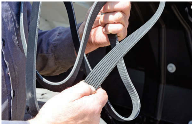
▲ Today’s serpentine drive belts are made of EPDM synthetic rubber that wears much like a truck tire. (Photo by Ed Wodalski)
