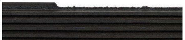
▲ A missing rib indicates it’s time for a new belt. (Photo courtesy Goodyear Engineered Products)
