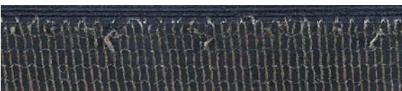
▲ Worn backing means this belt has reached the end of its service life. (Photo courtesy Goodyear Engineered Products)
