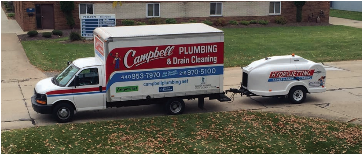
▲ Campbell's trailer-mounted Spartan Warrior water jetter (4,000 psi/18 gpm) made quick work of clogged lines that were threatening the operations of a local auto dealership.
