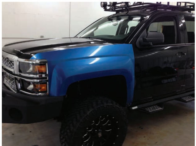
▲ Top photo: The brushed blue and gold WWETT Show truck began as a black 2014 Chevrolet Silverado 1500 4 x 4 extended cab; Bottom photo: Wraps are made from cast or calendered film and have a life span of up to seven years. Calendered film is best suited for flat applications, while cast easily negotiates the curves and contours of a front fender.
