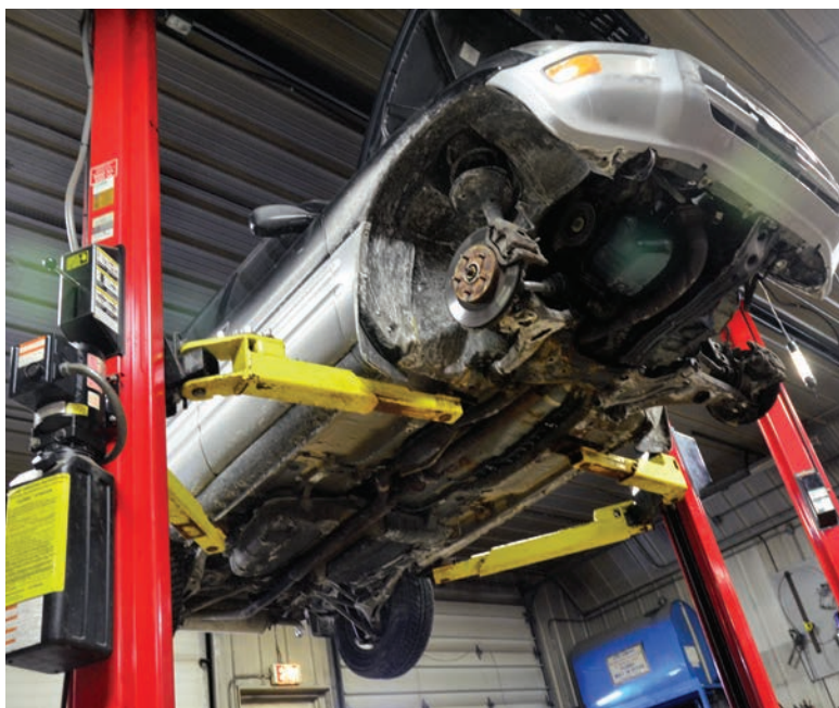
▲ Above-ground, surface-mounted lifts, typically bolted to the garage floor, are among today's most popular styles. (Photo by Ed Wodalski)
