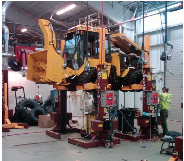
▲ Heavy-duty mobile column lift system. (Photo courtesy Mohawk Lift)
