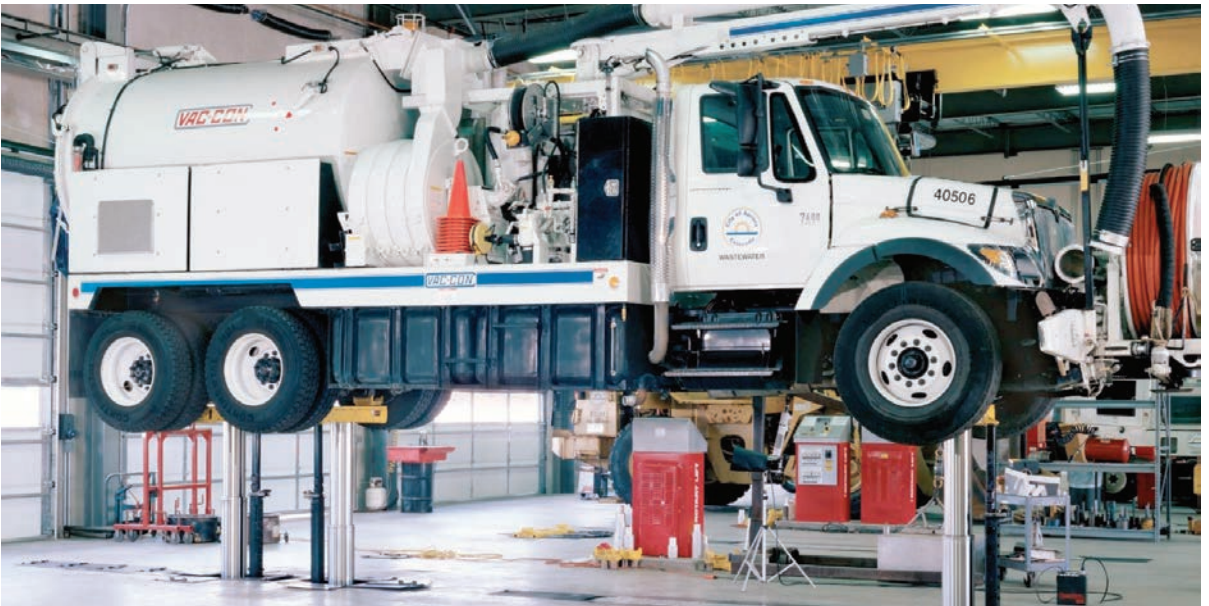
▲ Telescoping inground lift. (Photo courtesy Rotary Lift)
