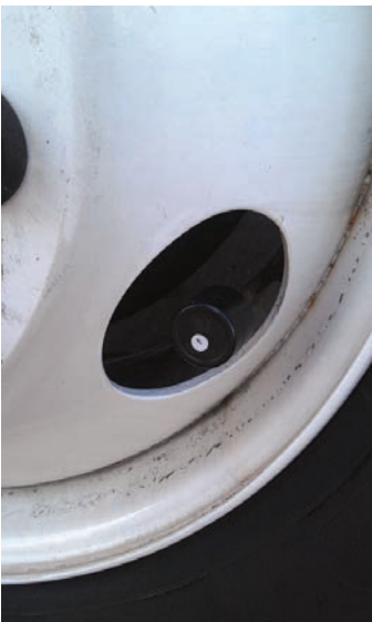
◀ A tire pressure monitor appears like a traditional tire stem at first glance, but is a high-tech gadget aimed at safety.
