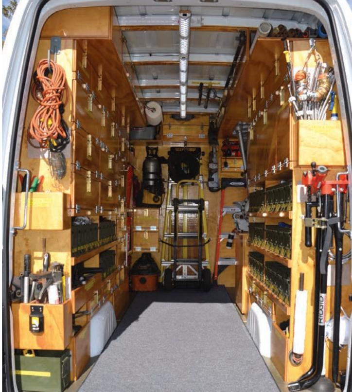
▲ The wide center aisle provides room for moving tools, equipment and storing temporary items, like water heaters. Illumination comes from four LED lighting strips, wired into the existing electrical system that powered the dome lights.
