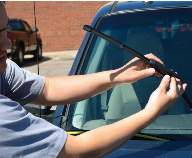
▣ Blade manufacturers recommend replacing your blades every six to 12 months, depending on climate and driving conditions. (Photos by Ed Wodalski)
