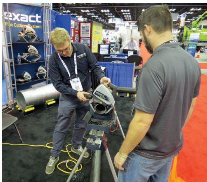
▲ Lauri Makkonen, a sales representative for Exact Pipe Tools, demonstrates the 170E saw for an attendee at the 2016 WWETT Show. The saw can cut any pipe material, including steel, copper, cast iron and all plastics .5 to 6.7 inches in diameter. (Photo by Luke LeNoble)
