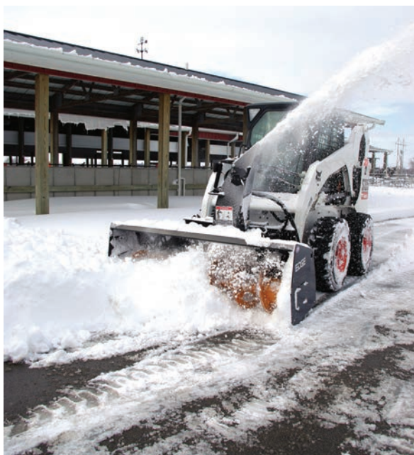
▲ Snowblowers can be a handy winter attachment. Before sending yours out in the cold, be sure to check the hydraulic hoses for cracks and wear and the condition of the cutting edge and skid shoes.
