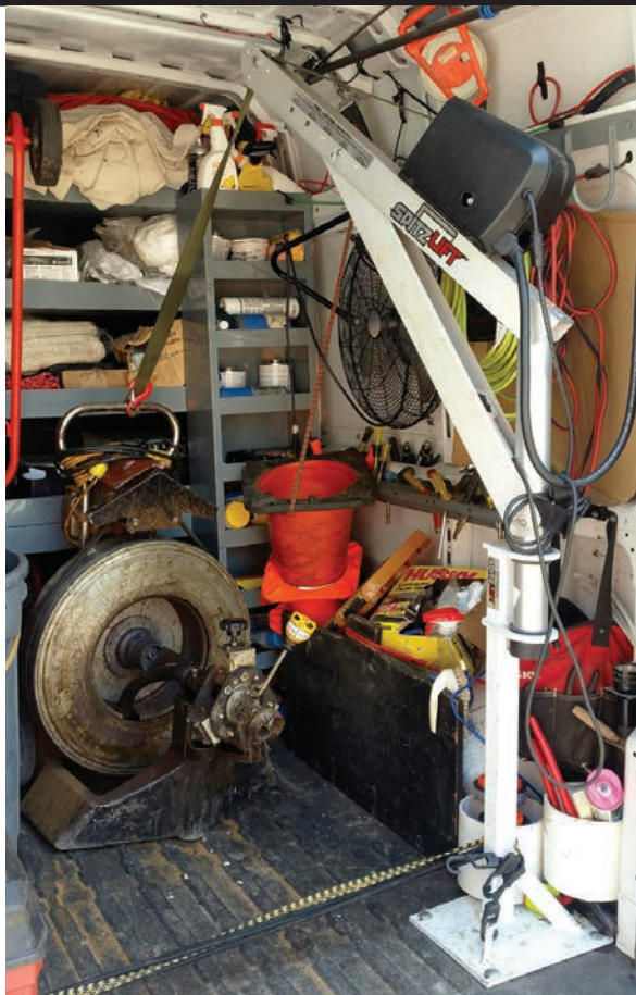
▲ The 40-pound aluminum hoist can lift up to 900 pounds.
