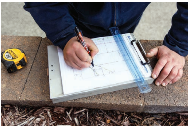
▲ Plumber Denny Kelley draws a map of a home for an inspection. The drawing is required in Lower Burrell, Pennsylvania, to show where the home connects to the city’s sewer system.
