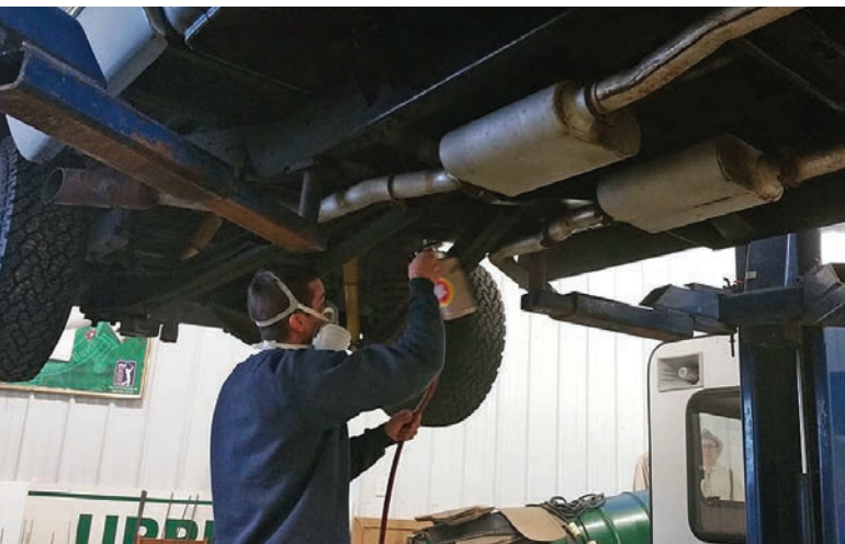
▲ Mike Stansbery, owner of Wyandot RustProofing, applies an undercoating of FLUID FILM, a lanolin-based rust inhibitor, to the undercarriage of a 1969 Chevy truck. (Courtesy of Wyandot RustProofing LLC)
