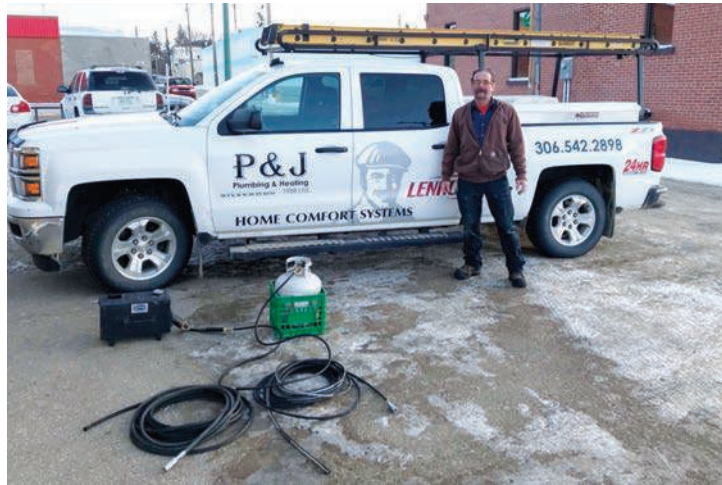
▲ Bruce Hunter, a plumber for 12 years at P & J Plumbing & Heating in Kamsack, Saskatchewan, stands near his service vehicle and an Arctic Blaster from Arctic Blasters. The Arctic Blaster is basically a water-boiling unit that heats water with a lit propane torch to create steam, which can then be led into a frozen pipe to thaw it. (Photo courtesy of P&J Plumbing)
