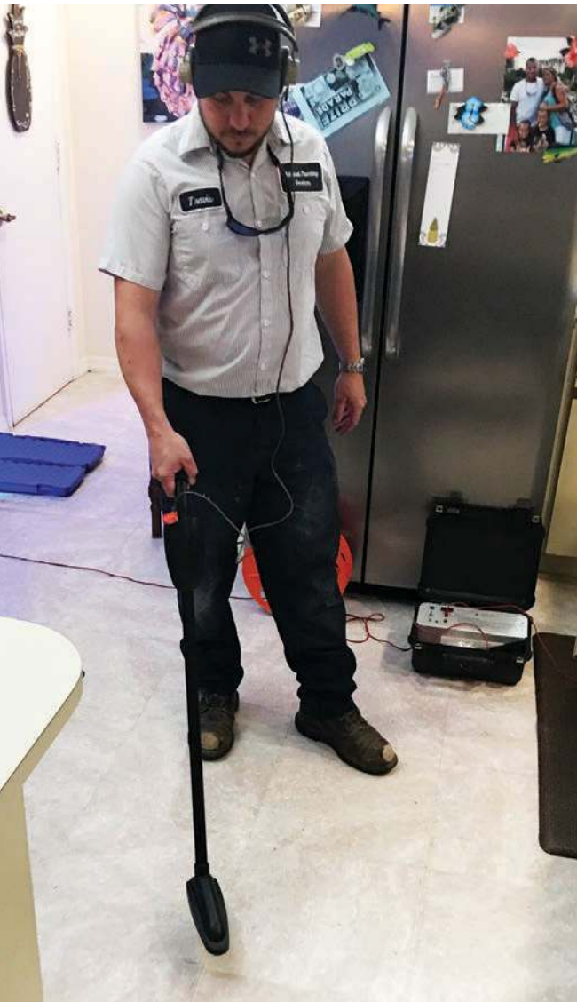
▶ Travis Nieves, Admiral Plumbing Services technician, uses Pulsar 2000 pipe-tracing and leak-detection equipment on a job site in Jupiter, Florida. (Photo courtesy of Admiral Plumbing Services)
