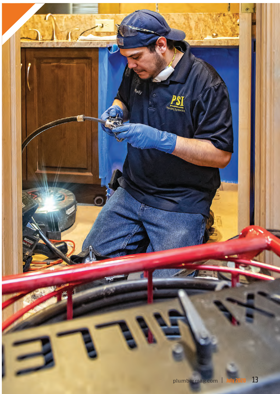
► Technician Rudy Frausto changes a chain knocker head on a Picote Solutions Maxi Miller prior to starting a drain cleaning job in a restroom at a commercial job.
