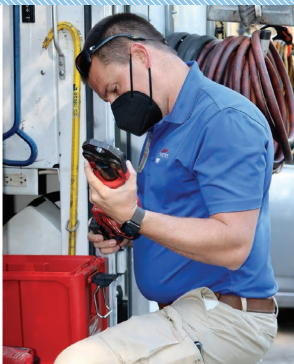
▲ Adam Westendorf, technician of Roto-Rooter Plumbers of Savannah, Georgia, prepares a copper press tool at a job site.
